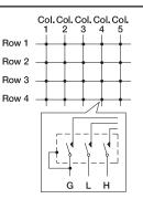
Each crosspoint in the matrix consists of a 3-pole Form A (normally open) relay. The shield of each relay is connected to the column GUARD line.
